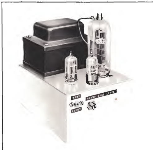
K2HAK's modulator employs TV-receiver type power transformer whose high-voltage secondary windings are designed to pass considerable current. Front of modulator shows "Mike Input" and slotted shaft for adjusting "Clamp Bias Level."
